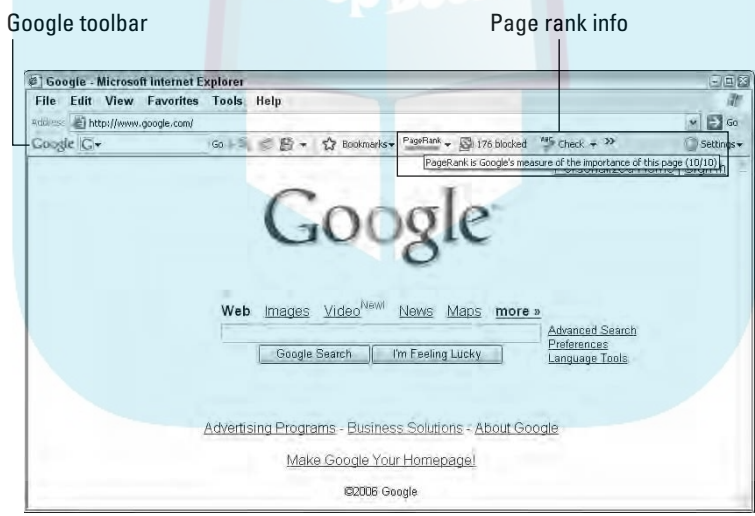
Figure 10-3: The Google toolbar shows PageRank with both graphics and text. Ranking is by page, not by site.
